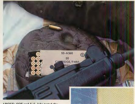
ABOVE: SOF and U.S. labs tested the latest Soviet body armor. UZI and ammo used in SOF tests rest on bullet-dented ballistic gelatin. RIGHT: Soviet vest components: titanium plate and four-ounce twill fabric contrast with light-colored Kevlar swatch.
